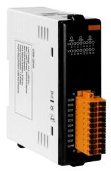
The USB-2045 is a full-speed USB device with 16 digital output channels module. The USB-2045 supports source type output and equips with short circuit protection. There are 16 LED indicators that can be used to monitor the status of the digital output channels. The 4 kV ESD protection, 4 kV EFT protection, 3 kV surge protection for power input and 3750 VDC Intra-module isolation are standard.
