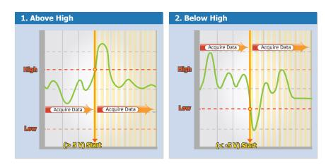
3. Leave-region: Trigger when the signal leaves the high and low level region, collect N data.
